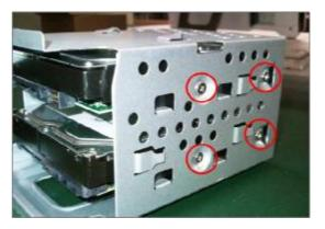
6.9 Put five hooks to Chassis and push HDD Cage down
